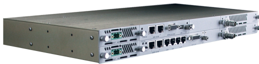
SkyWay-EM Signal Processing unit (SPU). Two radio modems can be loaded into a single SPU.
